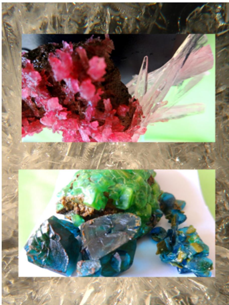
**Figura 2** Ammonium di-hydrogen phosphate with a pink food dye on a volcanic rock, showing different crystal habits; a mysterious green crystalline compound, from the reaction of copper (II) sulphate pentahydrate with potassium dichromate. The background of the slide shows tartaric acid crystals under the stereomicroscope, 10x.
